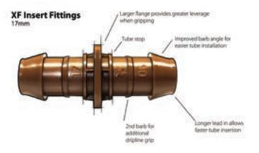
We recommend using the XF Insertion Tool (FITINS-TOOL) which lowers the effort required to insert each fitting by 50% (p. 142)
