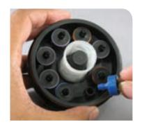
Helpful Hint: Always install emitters with the pointed end (inlet barb) or threaded end up, as shown
