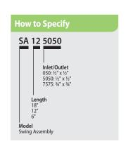
Swing Pipe Flexible Sprinkler Assembly
