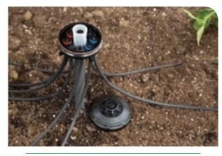
Each port can be configured on the Xeri-Bird™ by installing flow controlled emitters. Above shows a combination of 0.5, 1.0, and 2.0 gph Xeri-Bug emitters.
